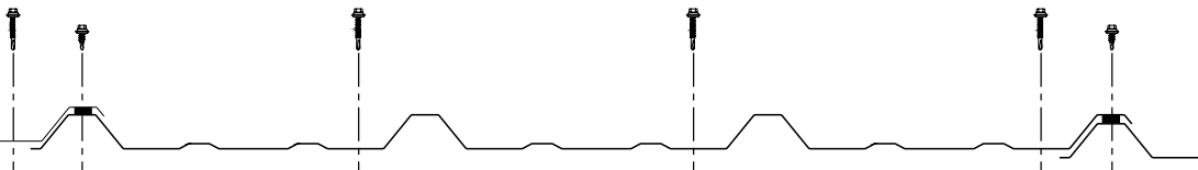
PBR-Panel Fastening Pattern - Interior
