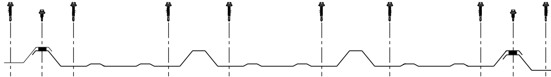
R-Panel Fastening Pattern - Ends
