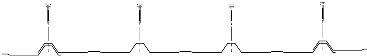
Typical Nail Fastening Pattern
